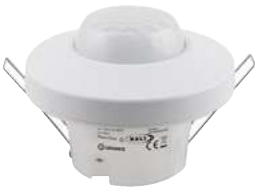
SENSOR DALI-2 LIGHT-PRESENCE-40X5 INFRARED CEILING INTEGRATION DALI-2 input device, infrared presence detector with 40X5 m movement detection
